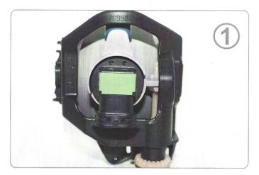
Find out the original halogen bulb position.
